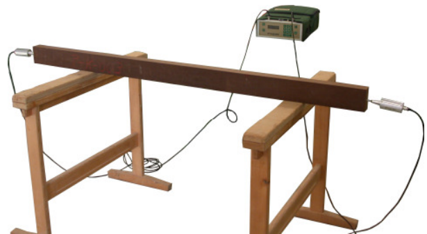
Figure 1: Determination of the longitudinal ultrasonic wave speed with the help of a "Sylvatest" device.
