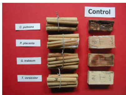
Figure 2: Comparative appearance of the reed bundles and the corresponding controls in accordance with Standard EN-113.
